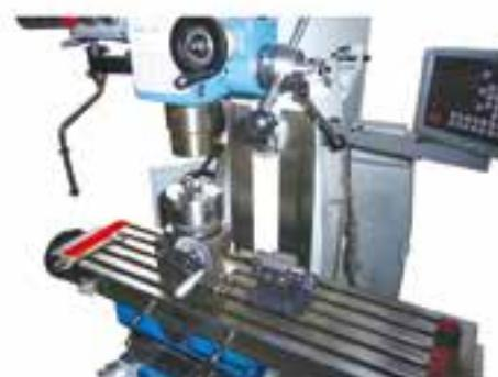
Rule: Divide 24 by the number of divisions required and the result equals the number of holes to move in the 24-hole rapid index plate. Thus,number of holes to move=24/D, where D is the number of divisions.
