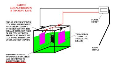
Connect the wiring as shown in the diagram above Install the ballast lamp supplied, into the socket on the power supply. The anodes hang from and are connected to the **black negative** rod. The item(s) to be stripped are suspended from and connected to the **red positive** rod. When the power is applied a stream of fine bubbles will be emitted from the anodes and illumination will be observed from the ballast lamp on the power supply.
