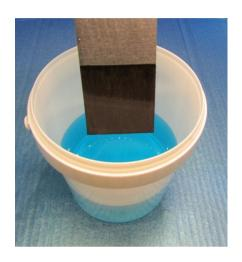
THE ZINC BLACK SOLUTIONS SHOULD BE CAREFULLY POURED INTO THE 2.5 LITRE BUCKET SUPPLIED. OBSERVE ALL SAFETY WARNINGS AND USE THE SUPPLIED SAFETY GLASSES, GLOVES AND MASK WHILST USING AND WORKING AROUND THE STEEL BLACK SOLUTION. AFTER USE STORE THE STEEL BLACK SOLUTIONS IN THE ORIGINAL BOTTLES FOR THE NEXT USE CLEARLY MARKED AS TO THEIR CONTENTS
