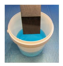
THE ZINC BLACK SOLUTIONS SHOULD BE CAREFULLY POURED INTO THE BUCKET SUPPLIED.
