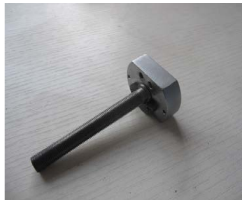
3. Assemble the block (Part No.8) and compound feed screw (Part No.6) on the bracket (Part No.2).
