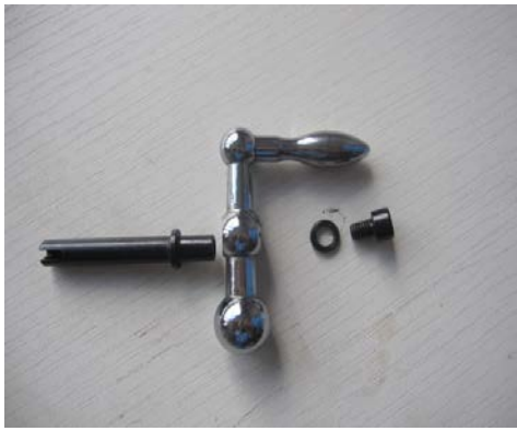
4. Assemble the transition shaft (Part No.4) onto the dismantled ball handle.
