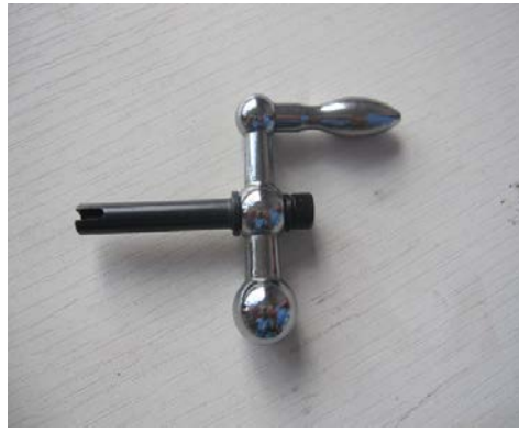
4. Assemble the transition shaft (Part No.4) onto the dismantled ball handle.
