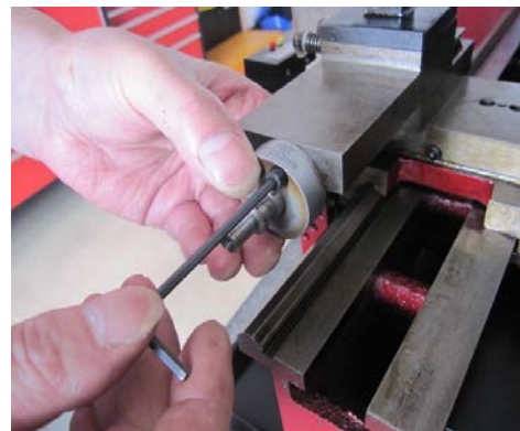
2. Loosen the screws. Remove the dial bracket, and take out the compound feed screw dial.
