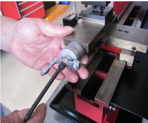
1. Remove the screw securing the compound handle. Remove the ball handle, spacer and dial.
