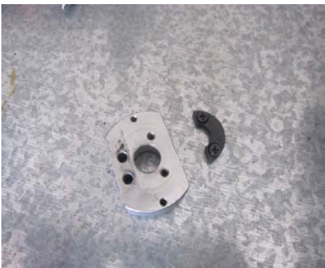
3. Assemble the block (Part No.8) and compound feed screw (Part No.6) on the bracket (Part No.2).
