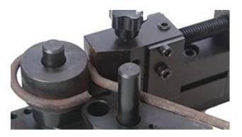
Choosing corresponding specifications of the circle, keeping the workpiece between activity block and circle, loosen the handle after rotating the handle to the right angle, moving the workpiece clamping point then to rotate handle step by step, until the ring form as shown in figure.
