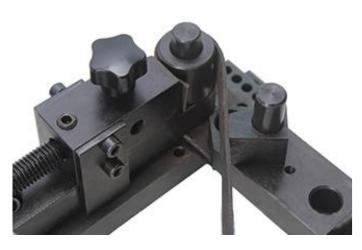
Choosing a appropriate circle and angle module, catching a sheet end between them, loosen the handle after rotating the handle to the right Angle, move the workpiece clamping point to rotating handle, step by step, until the ring form as shown in figure. We can transform clamping points, bend the workpiece of any shape.
