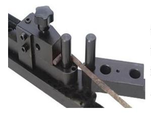
Using two 13-mm shafts, keeping the bending workpiece between block and fixed axis, then rotate the handle a quarter circle, a 90 °circle arc lasts.
