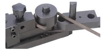
According to the size of the workpiece to select the size of the circle, the circle material can be half a circle, circle, arc curved shapes such as bending.
