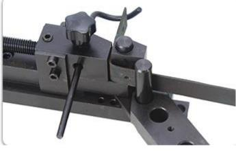
Using a appropriate angle module , adjusting the set rule to the appropriate size, clamping workpiece as shown, which can bent square workpiece, increase work efficiency and the accuracy of the workpiece.
